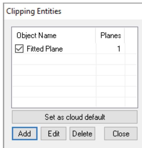
Clipping planes are defined per cloud through their properties, allowing a user to define a separate clipping plane or set of clipping planes per cloud. We have now expanded on that for the simple case where an operator wants to use the same clipping plane for multiple clouds. To do so we have added the option to define any particular clipping plane configuration as the system default, such that each additional cloud inherits the defined global clipping plane(s).
